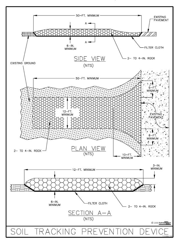
Figure V-19: Illustration of a Soil Tracking Prevention Device
